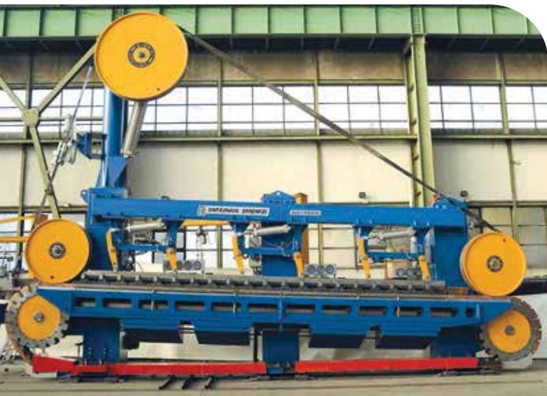
Continuus-Properzi Track & Belt Line and Typical Properzi Ingots/Bundles
