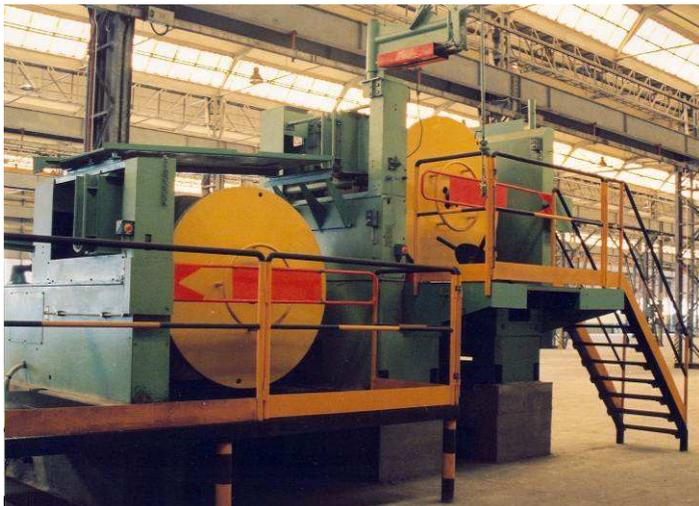
**Figure 14 – view of an automatic twin reel coiler**
