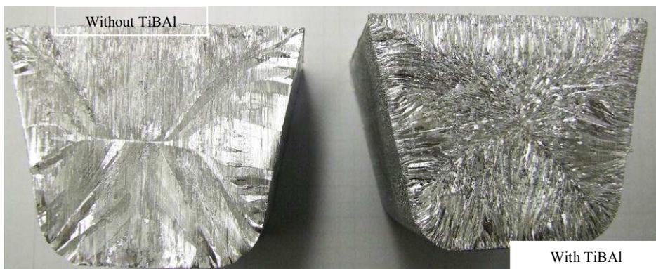
Figure 9 – cast bar cross section area
