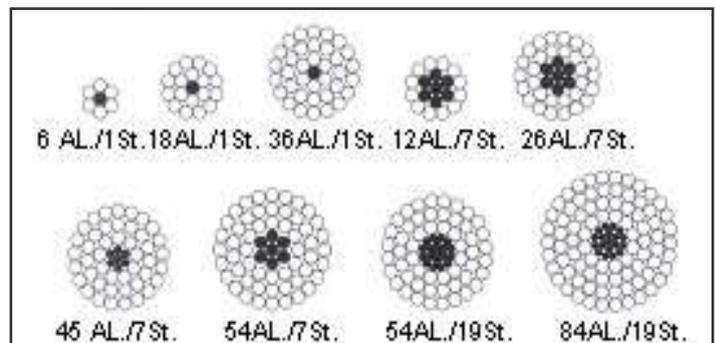
Fig. 3 – Typical ACSR Conductors
