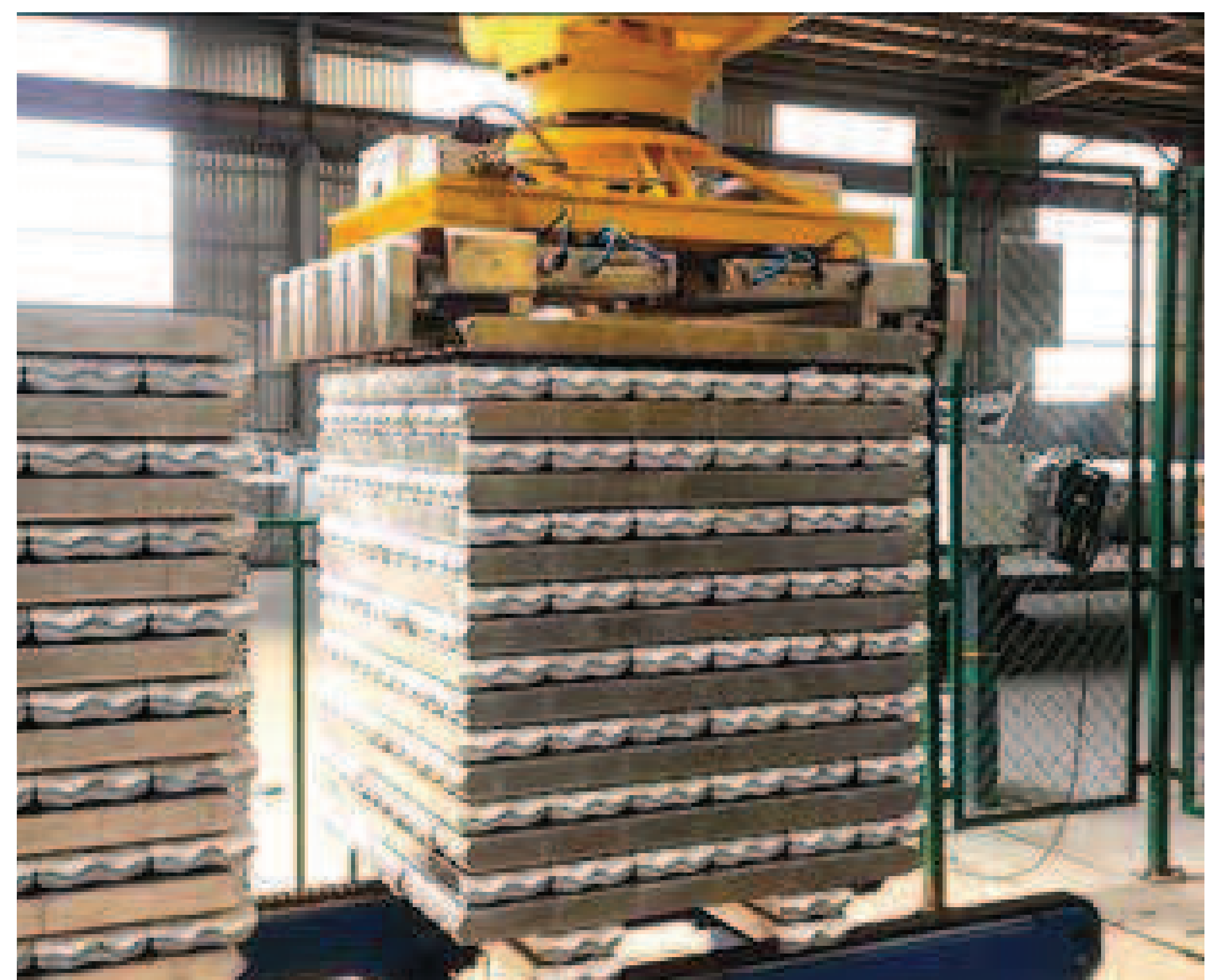
Properzi ingots during bundling phase.
