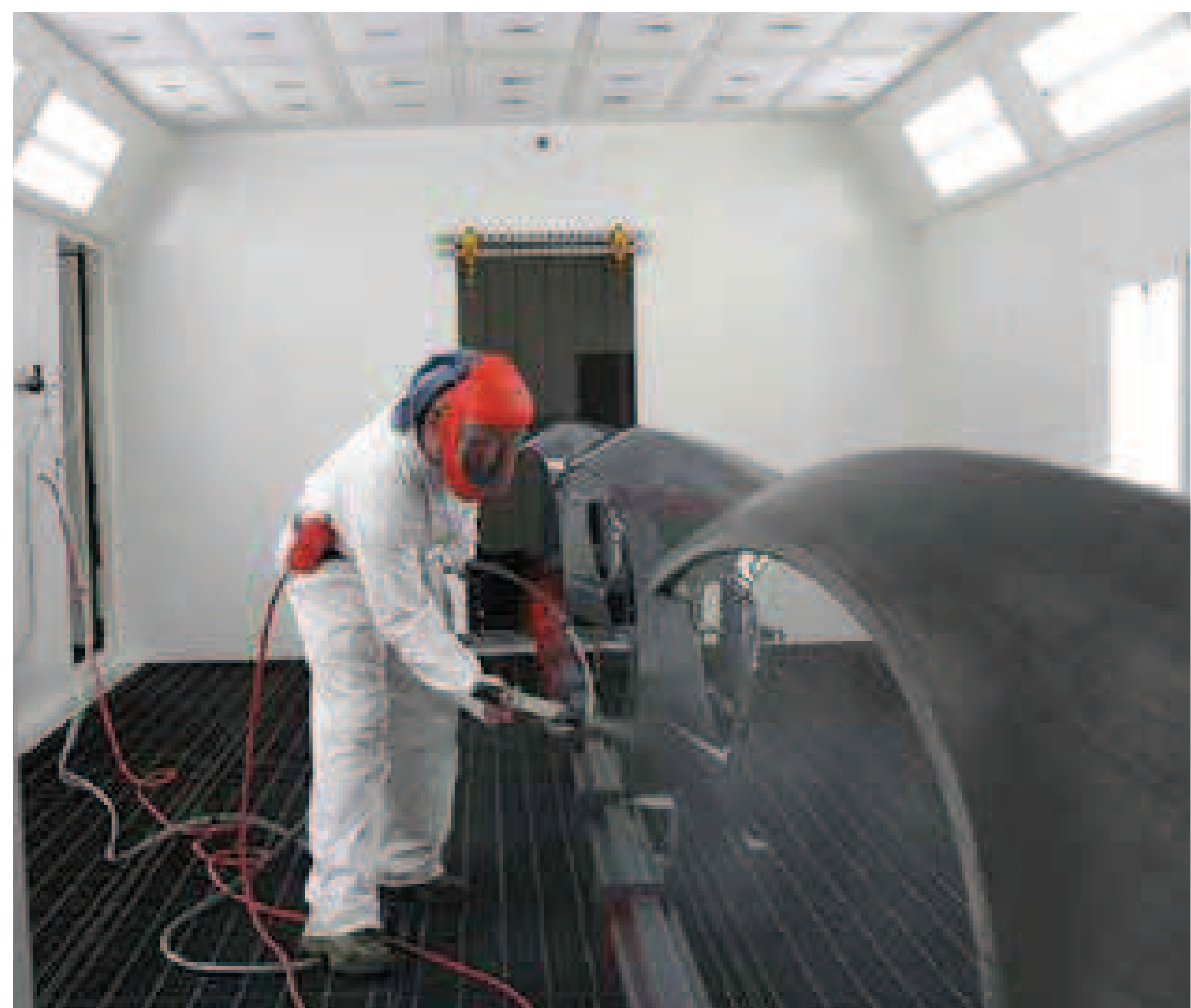
Zinc coating application by spraying method.
