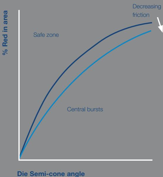
Figure 2 – Schematic curve illustrating the relationship between reduction in area during wire drawing and the corresponding die semi-cone angle
