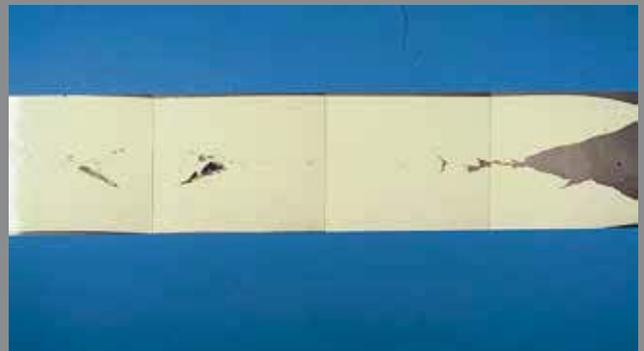
Figure 4 – Photomicrograph illustrating wire cracks pointing in both directions
