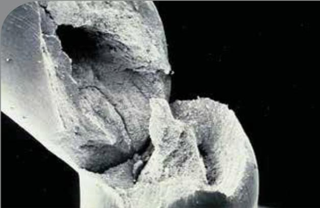
Figure 1 – Typical cuppy wire break
