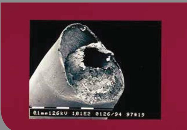
Figure 5 – Cone break initiated by macroporosity
