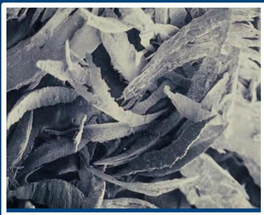
Figure 1 – typical fines that are produced by abrasive wear
