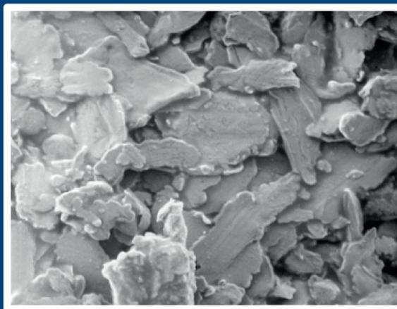
**Figure 4 – fines resulting from delamination wear**
