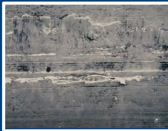
Figure 2 – adhesive wear between two copper wires making contact with each other during drawing
