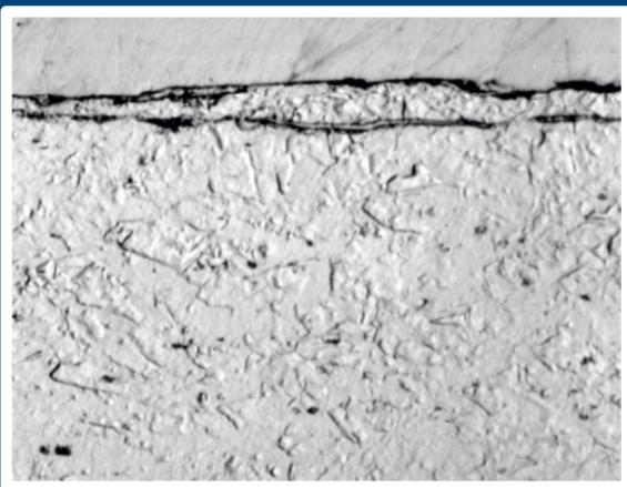
**Figure 3 – transverse wire section showing subsurface tensile cracks leading to subsequent delamination wear fines**
