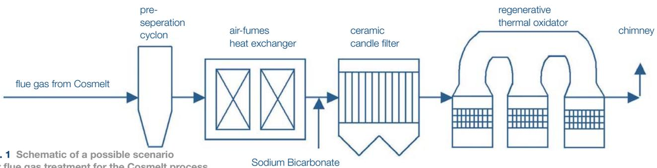
**fig. 1** Schematic of a possible scenario for flue gas treatment for the Cosmelt process.
