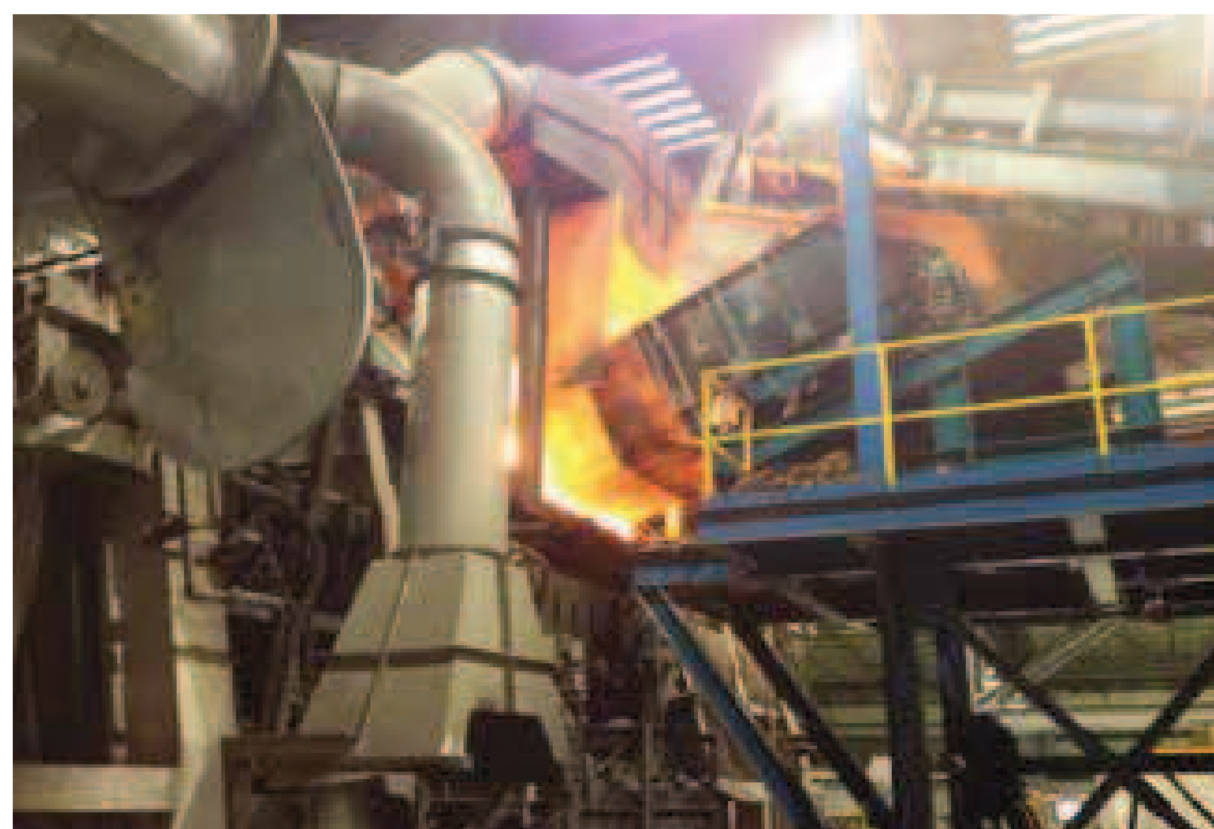
Scrap loading from the top of the furnace.
