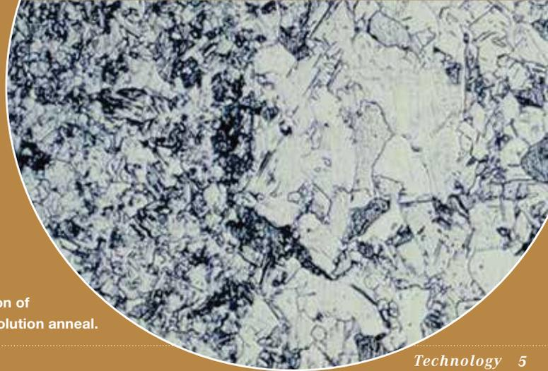
Duplex microstructure caused by dissolution of copper oxides during a high temperature solution anneal.
