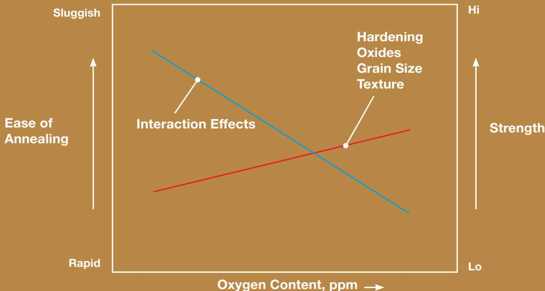
Schematic representation showing the effects of oxygen content upon annealing behaviour and hardening of copper.
