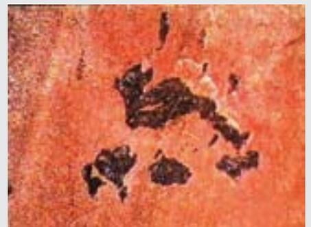
Figure 2 - Subsurface oxides on the alcohol deoxidized ETP copper rod
