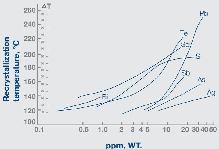
Figure 1 - Effect of impurities upon annealing temperature of high-purity tough-pitch copper
