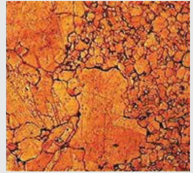
Photo 3 - ETP Cu, Ø 8.00 mm: hydrogen embrittlement within the copper structure, after hydrogen atmosphere annealing
