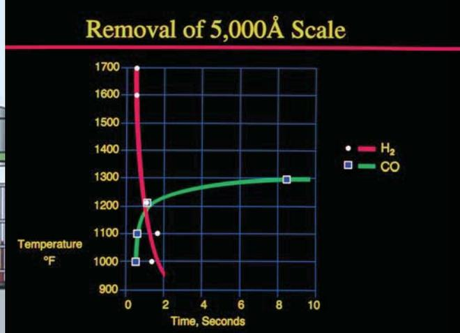
Removal of 5,000 Å oxide diagram (temperature/time)
