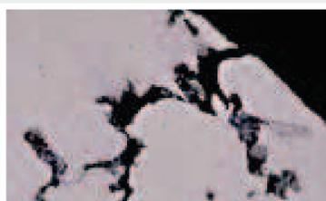
**Figure 1** - Hot cracks that formed in the copper matrix grain boundaries of the as cast bar due to excessive tensile stresses, thereby resulting in subsurface oxides
