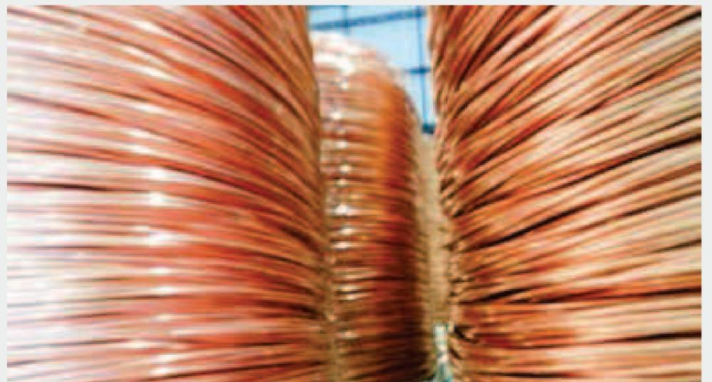
Copper rod coils before break-down operation
