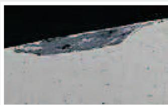
**Figure 2** - Typical exfoliated copper oxide particle re-embedded in the rod from inadequate high pressure descaling
