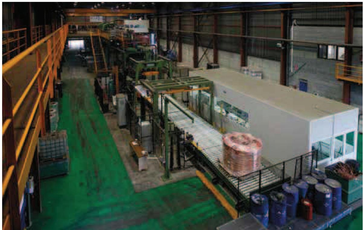
*Automatic Packaging Line of a 25 tph Properzi Rod Plant.*
