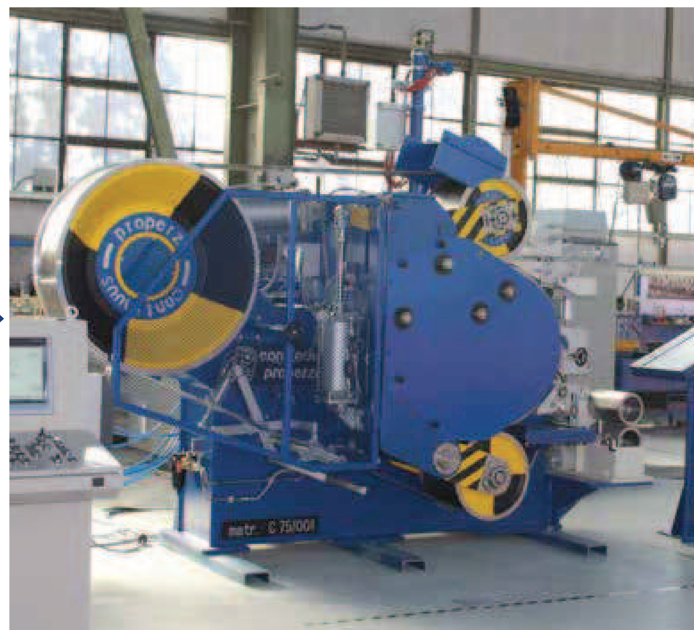
Latest Properzi Casting Machine for the production of wide Pb Strip.
