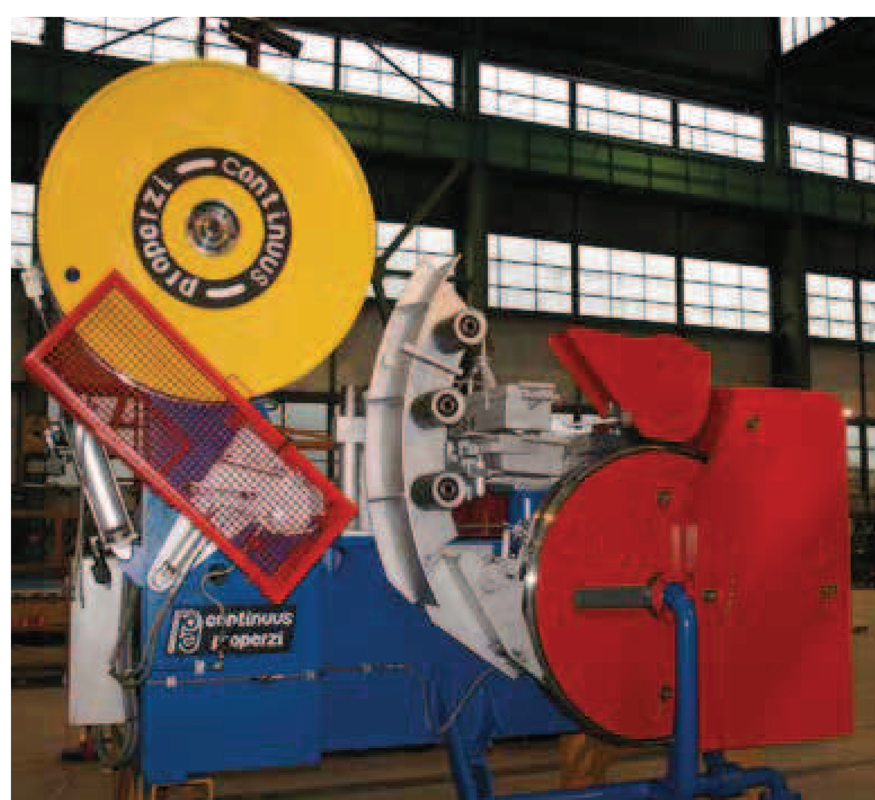
Properzi Casting Machine for the production of narrow Pb Strip.
