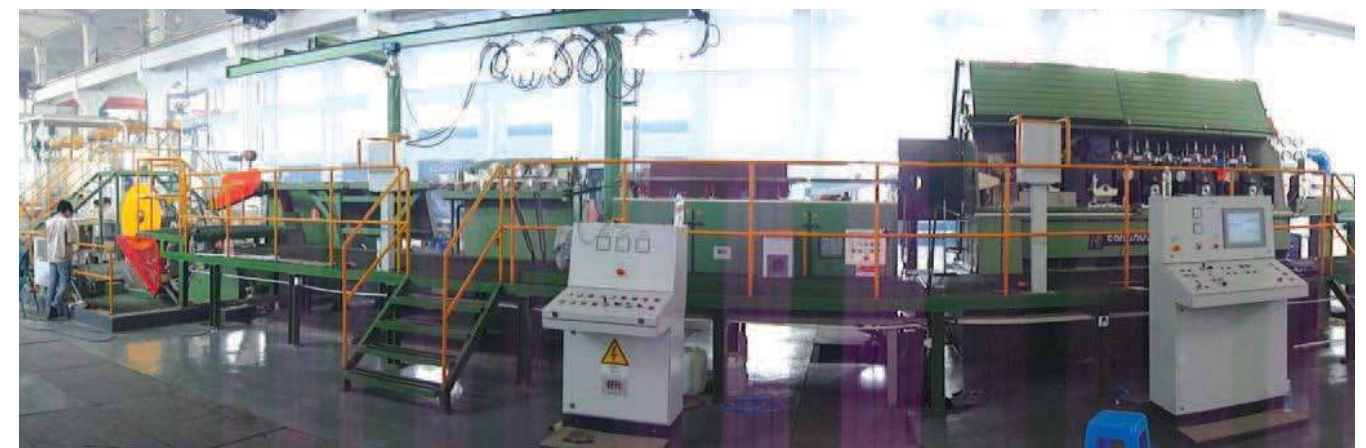
Propenzi CCR (Continuous Casting and Rolling) Aluminium Line.
