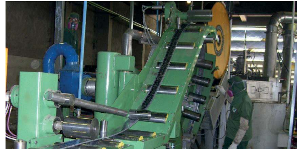
Pb Strip Conveyor.
