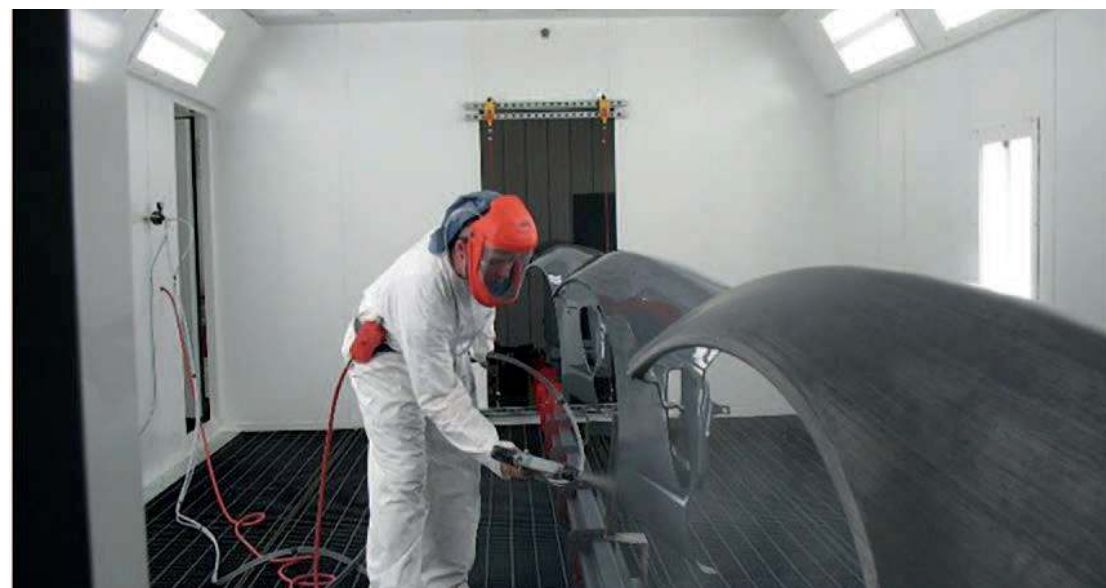
Zinc coating application by spraying method.
