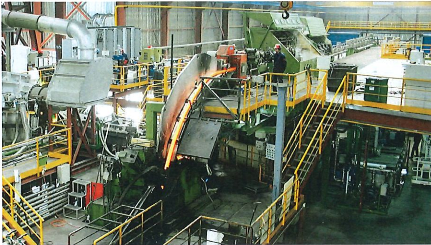
Modern CCR Copper Line from Furnace set to automatic coiling system
