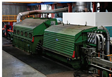
Modern Rolling Train for aluminum – Roughing Mill + Finishing Mill (top) and Modern Rolling Train for copper – Roughing Mill + Finishing Mill (at right).
