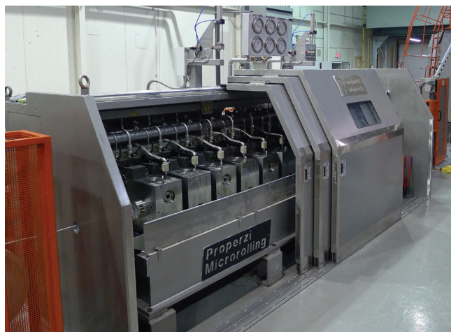
Modern Properzi Microrolling® Mill .
