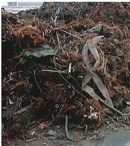
Copper scrap of lower quality - 94-99% Cu
