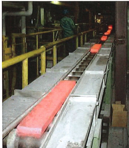
Properzi CU Ingots after the Rotary Shear
