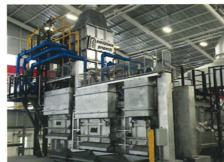
Properti Vert-Melt Furnace in operation at 5 tph rate EC Rod. Photo: Properti
