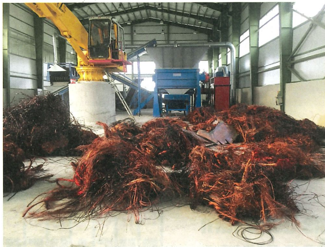
Fig. 4 — The Vert-Ref furnace set is fed with scrap having a copper content of \geq 97\% .
