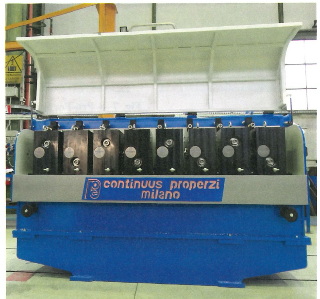
Fig. 6 — Self-Annealing Microrolling® (SAM) method.
