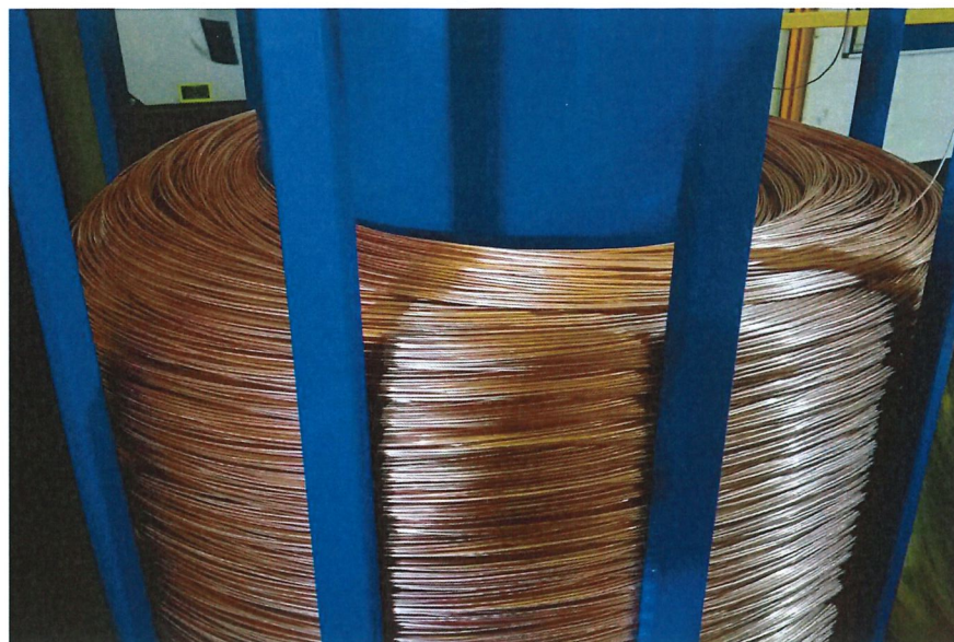
▼ Copper wire obtained with Properzi's self-annealing method
