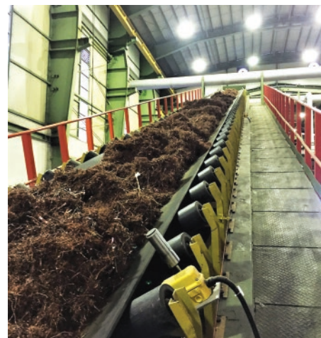
Conveyor belt feeding copper scrap to a 250-ton top-loading reverberatory furnace. Photo: Properzi
