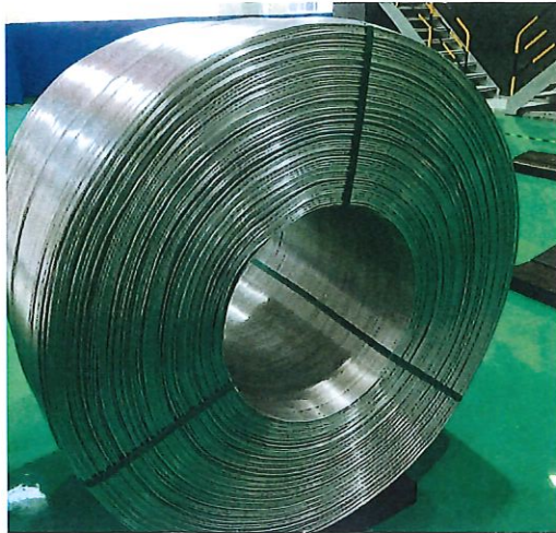
Tight coil of 6 mm diameter wire continuously cast on the CCW Line
