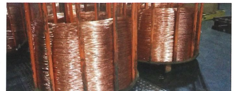
Copper wire obtained with Properzi SAM. Photo: Properzi
