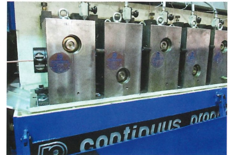
Passage of the rod in the Properzi Microrolling® Mill. Photo: Properzi
