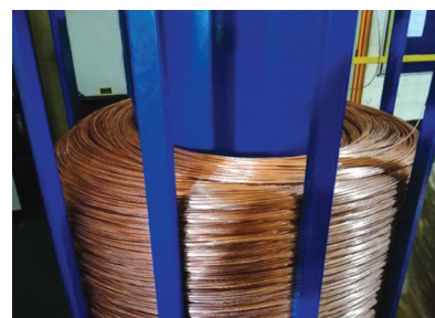
Fig. 2 — Soft Cu wire using the Properzi Self-Annealing Microrolling (SAM) process.
