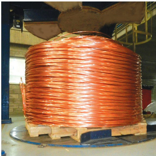
Aluminium rod produced with Properzi technology (above), and copper rod produced with Properzi technology (below).
