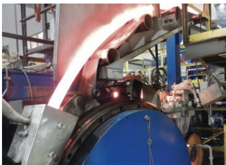
1 Properzi Casting Machine. Photo: Properzi
