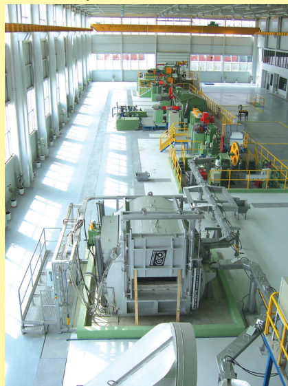
Typical Properzi Aluminium CCR Line.
