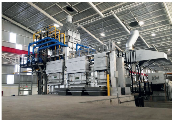
Figure 2. The Vert-Melt in operation: The Static Holder in front, the Tower Behind
