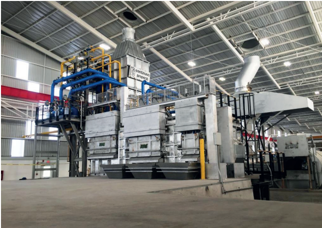
Fig 2. The Vert-Melt in operation: The Static Holder in front, the Tower Behind
