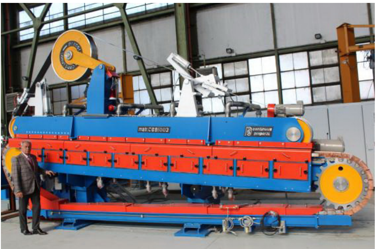
The track & belt machine for the production of CO 2 ntinuous Green Ingots.
