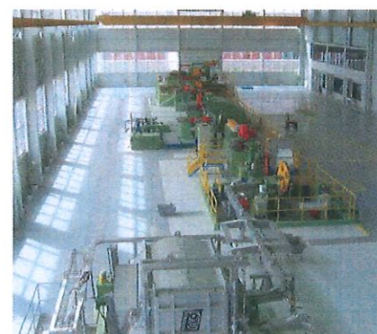
Example of a CCR aluminium line for internal consumption by cable producers
