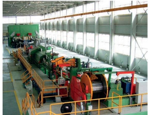
A Typical Properzi Continuous Casting and Rolling Aluminium Line
