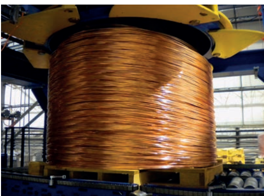
A Copper Coil Produced, Using Properzi Technology
