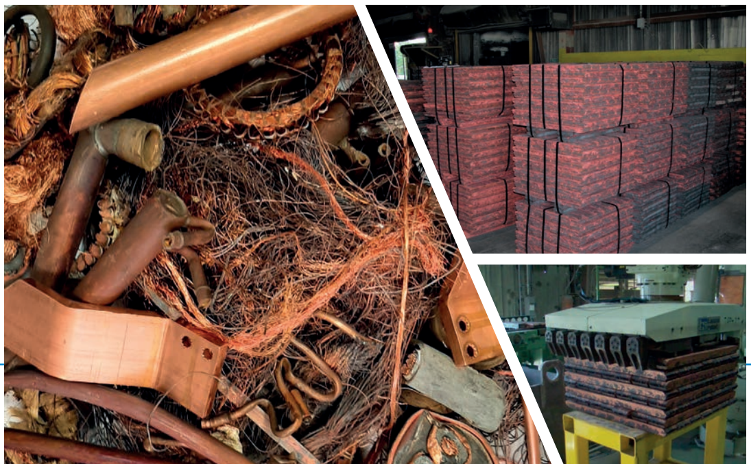
Properzi Copper Ingots, Obtained from Recycled Scrap
